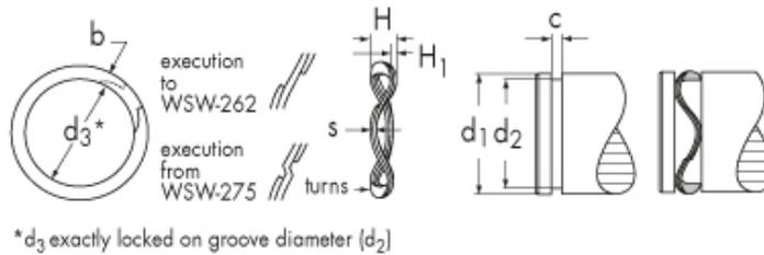
\*d<sub>3</sub> exactly locked on groove diameter (d<sub>2</sub>)
