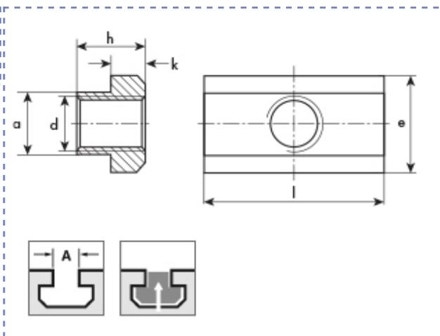
T-slot nuts, T-slot nuts profile
